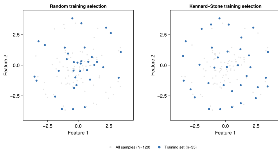
Figure 1: Random and Kennard–Stone training-set selection on a synthetic dataset with a dense centre and a sparse boundary. Gray points denote all samples ( N=120 ) and blue points the training set ( n=35 ). Kennard–Stone covers the boundary of the experimental domain, whereas random selection concentrates in the centre.
