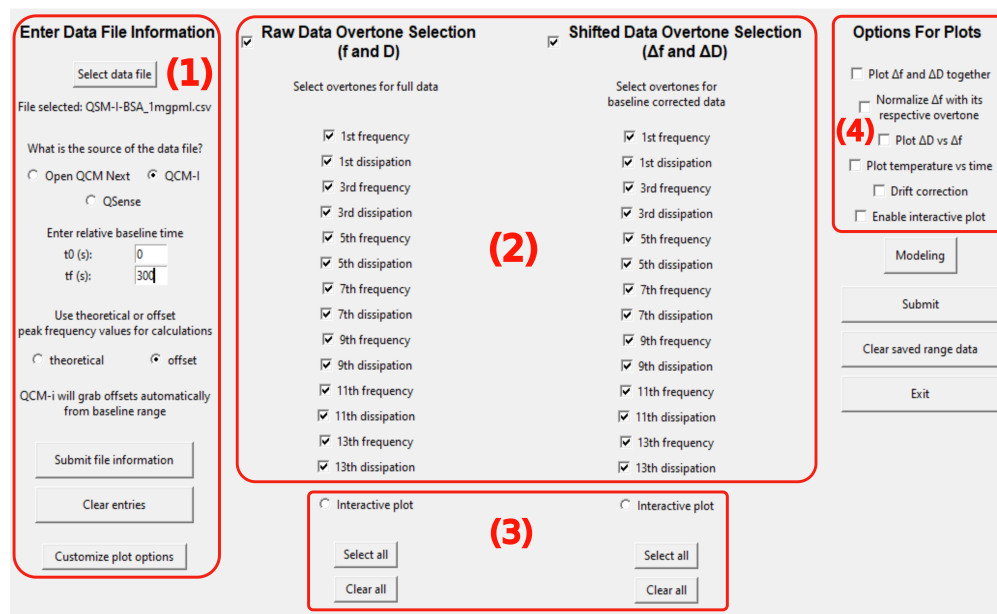
Figure 1: User interface of pyQCM-BraTaDio. (1) Initialization conditions, (2) selection of frequencies and dissipation for data mining, visualization, and modeling, (3) interactive plotting options for data range selection, and (4) selection of plotting options and modeling.
