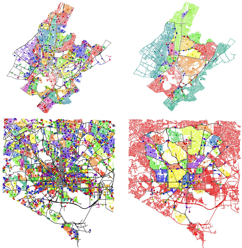
Figure 1: Automated generation of Superblocks. Athens, GR (top row) and Baltimore, MD, USA (bottom row) Superblocks generated using the residential partitioner (left column) and the betweenness partitioner (right column). Each Superblock is plotted in a different color, the rest of the streets are black. For easier visual recognition, each Superblock is also highlighted by a representative node of the same color. Map data from OpenStreetMap.
